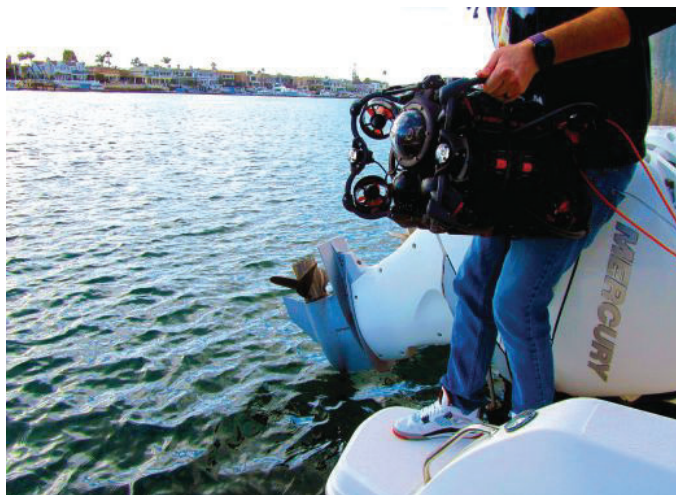
» The SRV-8 is powered by two lithium-ion batteries that allow for 6 to 8 hours of operation and its size allows for one-person portability. (Photo credit: RJE Oceanbotics)
