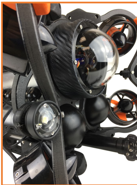
8 Thrusters, Dual-Mode Camera, 130° Beam Angle Lights, 3,000 Lumens Each
